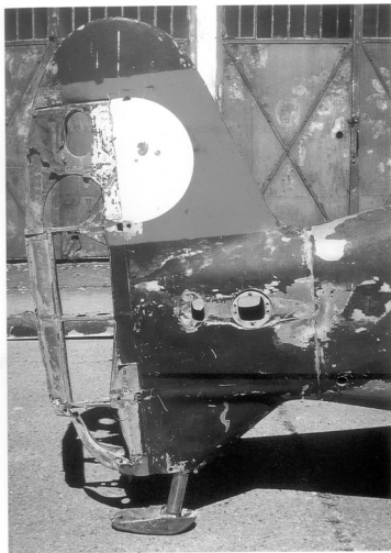
The starboard side view of the Me 209 V1 's tailplane section. It is a mirror image of the port side except that it carries no werks nummer . The bulge in the ventral portion of the tail fin seen between the horizontal stabilizer and the metal tail skid was required to allow linkage sufficient space when moving the rudder.
