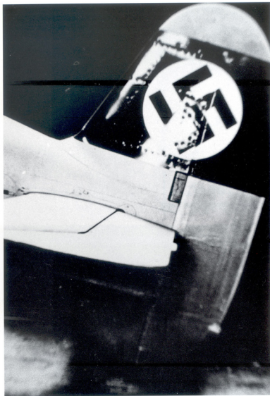
The Me 209 V2's tail assembly and featuring its vertical stabilizer's elevator trim tabs. This machine has the Hakenkruz (swastika) in red applied within a black band on the upper portion of the vertical stabilizer.
