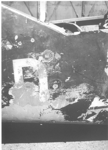
Direct side view of the aft cockpit of the Me 209 V1 as seen from its starboard side. Two access ports are visible. The upper is an electrical receptacle (outlet) for taking an external 24 volt power line while the aircraft is on the ground. The purpose of the lower access port is unclear.
