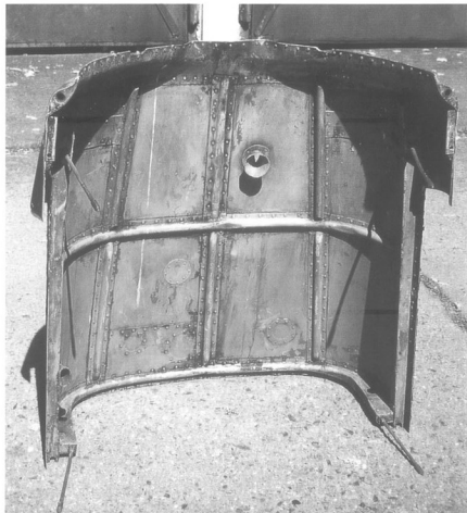
The inside appearance of the cowling covering the underside of the Daimler-Benz 601 racing engine. It appears to be in remarkably good condition. The long rods at each corner are needed to go between the exhaust stacks and reach the upper cowling where it is secured. The circular item seen is a vent, allowing the escape-ment of water vapor/steam from the engine's cooling system.
