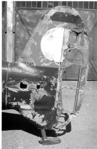
The port side view of the Me 209 V1 's tailplane section. The fabric has disappeared from the rudder but otherwise the tail assembly looks in very good condition for being in storage for over sixty years. The hydraulic metal tail skid appears to be in good condition as well. Notice the machine's werks nummer painted on the vertical fin... W.N. 1185 . Two openings can be seen in the tail assembly. The first is where the vertical stabilizers are bolted on to the fuselage. The second opening is where the actuating arm moving the elevators enter the fuselage. There is no trace of the Halkenkruez ( swastika ) within the white ball where it once appeared having been painted over.
