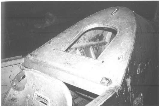
The rear cockpit-area of the Me 209 V1 as seen from its port side. The three metal brackets were hold-down mountings for the rear part of the cockpit canopy. Notice that the area behind the access port has been illuminated by the flash camera. The pilot's seat back has suffered a gash on its starboard side coming from the air raid on the Berlin Aviation Museum where the machine had been on public display.
