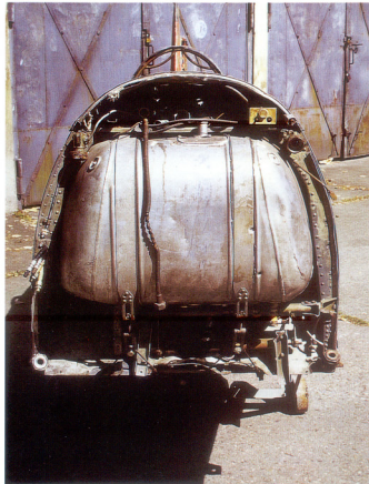
A close-up view of the Me 209 V1's aluminum insulated "cool stuff" tank, its hold-down metal straps, and plumbing. Notice to the far left and about center in the photo can be seen a bundle of cable ends which then lead back into the cockpit. To the far right and center in the photo can be seen an attachment device for the fuselage side cowlings. At the bottom of the fuselage can be seen two large diameter holes. This is where the cantilever engine mount's lower arms were bolted on to the fuselage. Where the port upper arm bolted onto the fuselage can be seen just above the "cool stuff" tank. It is seen as a large round hole in the upper right side of the photograph. The long dark cable appearing on the left side of the "cool stuff" tank with a connection at its end is the cable coming from the engine to the cockpit for the mechanically-driven engine revolution counter.
