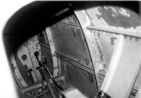
A view from the seat back access port into the aft area of the fuselage. The linkage seen here, above the jacking support bar, is for the elevators (top linkage) and for the rudder (lower linkage).
