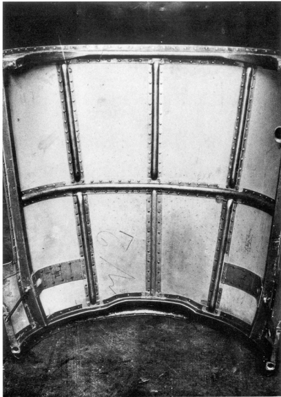
A piece of lower fuselage cowling for the Me 209 V2. This author does not know where it fits on the V2's fuselage.
