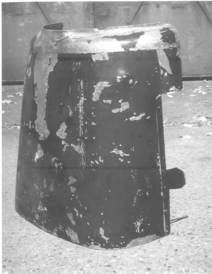
The port side view of the under engine cowling/cover shown placed on its aft end. Notice the long, steel rod used to align and help secure the cowling. There were four such long, steel rods on this cowling, one at each corner.
