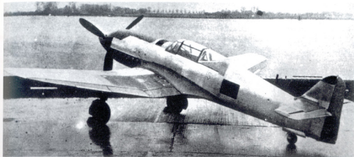
The Heinkel He 100 V1 shown here without paint, national markings, or code numbers. It was first flown on 22 January 1938, and later, in March 1938, was sent to E-Stelle Rechlin for further testing. This machine's engine was cooled by wing surface evaporation, and while at Rechlin was test flown by General Ernest Udet to an unofficial FAI Absolute World Air Speed Record of 394.2 mph, thus bettering another unofficial world air speed record held by the Italian Nicolot by more than 50 mph.
