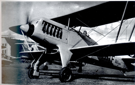
The Heinkel AG bi-wing He 51. It was put into Luftwaffe service in 1933 with a maximum speed of 200 mph and a service ceiling of 25,000+ feet. It was usually armed with 2xMG 17 cannons. After the Bf 109 replaced it about 1938, the old bi-wing still served, although as a trainer. Approximately 700 He 51 machines were manufactured between 1933 and 1938.
