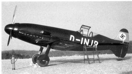
The cockpit canopy of the Me 209 prototypes each lifted and opened to their starboard side...typical of the Messerschmitt Bf 109s. Scale model and photograph by Günter Sengfelder.
