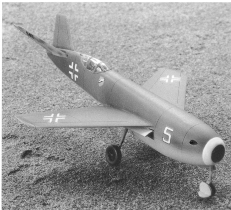
The long nosed Messerschmitt Me P.1106 with its butterfly tail and featuring its starboard side. It was to have been powered by a single Heinkel-Hirth HeS 011 turbojet providing 2,866 pounds [1,300 kilograms] of thrust. Scale model and photograph by Dan Johnson .
