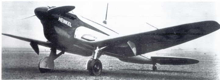
The loser in the RLM's mono wing fighter competition...the Heinkel He 112V1. It was destroyed on 15 April 1936 when it entered into a flat spin and its pilot Gerhard Nitschke bailed out. The V1 is shown here with its two-bladed HKW (Heidenheimer KupferWerke) propeller.
