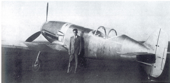
A dapper-looking Dr.-Ing. Hermann Wurster in suit and tie stands at the Me 209 V1's port side wing root of that "little monster," as he lovingly called it. The small oval opening on the wing's wing root by Dr. Wurster's right hand is the air intake for the steam to water condensing radiator. Another opening was on the opposite side.
