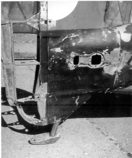
A close-up of the hydraulically retractable metal tail skid pad as seen from its port side. The skid pad was extended by compressed air and oil. Upon close inspection it appears to be in relatively good condition.
