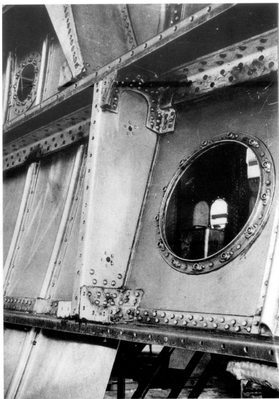
The inner side of the upper surface wing panel on the Me 209 V4. This author does not know the purpose of the large round port hole and why it was placed in this area.
